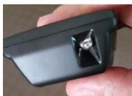
The end of the remote control has an Infra-Red transmitter that transmits the signal, which is invisible to the human eye, but if you pick up your 'smart phone' with a camera, turn on the camera and point the remote transmitter at the camera, push a button on the remote and see what happens. You should see the transmitter flash. You don't have to take a pic, just watch the screen.
